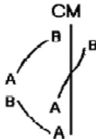
The Arc to Chord correction then corrects the grid bearing to a plane bearing. The nomogram of Arc to Chord Correction will supply correction values of sufficient accuracy for many applications and shows that surveys of limited extent (say less than five kilometres) and requiring lower precision may be able to ignore the correction.
